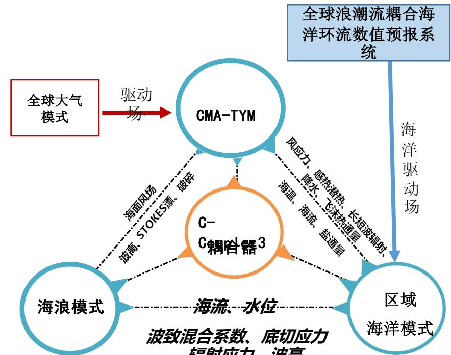
Schematic diagram for the regional air-ocean-wave coupling model
