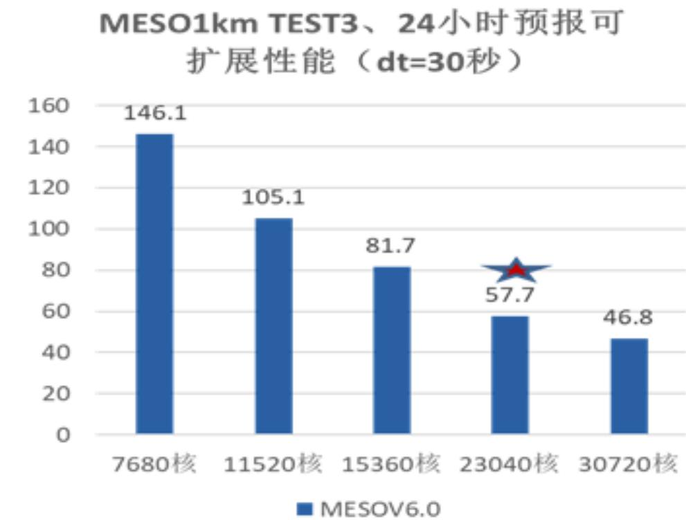
TEST2 - scale 3301x3301x70 (: TEST3 - scale 7501x5001x70. 2. New machine + optimization, the computing efficiency of the 1-kilometer eastern area of the regional mode is increased by 50%; 1 km national area uses 23040 nuclear 24-hour forecast to complete within 1 hour
